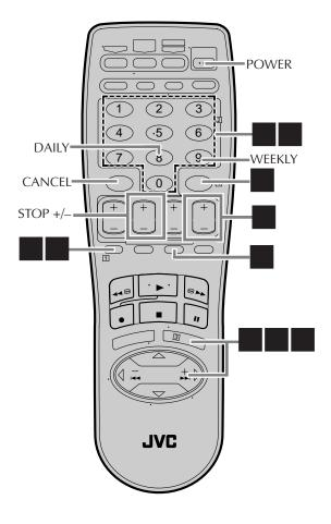
Timer recording allows you to program the VCR to automatically record a broadcast at some future time. Up to 8 timer recording programs can be made using VCR Plus+ timer programing or Express timer programing method (127 pg. 28) as far as a year in advance.
