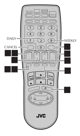
You can directly program the VCR's timer to record up to 8 broadcasts, as far as a year in advance. Remember, the clock must be set before you can program the timer (pg. 8 or 10).
