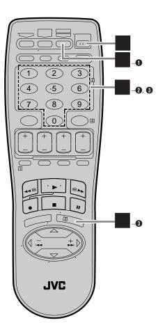
This Remote is capable of transmitting two control codes; one set to respond to A code control signals and another set to respond to B code control signals. This Remote control is preset to send A code signals because your VCR is initially set to respond to A code signals. You can easily modify your VCR and the Remote to respond to B code signals.
