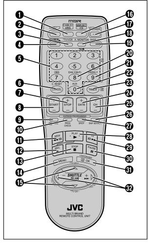
Buttons with a small dot on the left side of the name can also be used to operate your TV while holding down **TV** on the Remote. (**EP pg. 38**).
